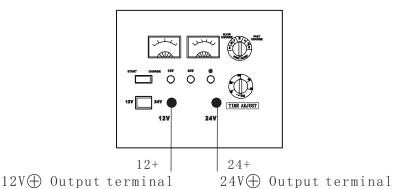
NB! Unplug the charger from the mains before you connect up the battery to the charger.
