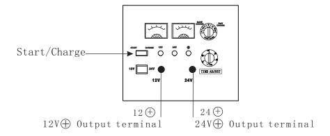
NB! Unplug the charger from the mains before you connect up the battery to the charger.
