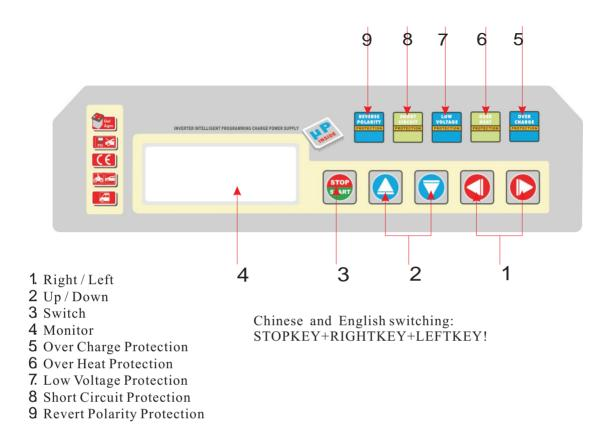
Overcharge Protection: In the charging process, the machine will constantly detect the battery state to see whether the charging is finished to prevent damage from overcharging.
