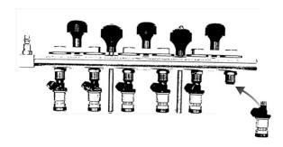
7..Please plug the pulse wire with the injector socket in sequence according to the numbers on the pulse wires
