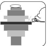
8.Starting up the fuel pump, turning the functional knob clockwise to adjust the pressure. If there is any leakage on the connection, please find out the reason and reinstall.
