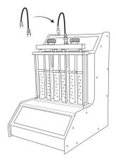
6.. Mount the injectors to the fuel stage.
