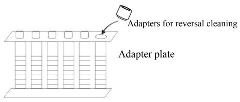
2. Connect injectors with suitable adapters. The injectors should be mounted in up-side-down.
