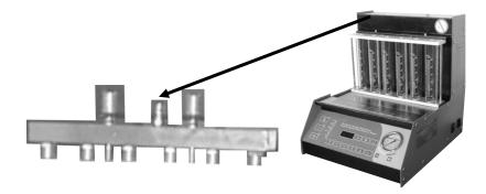
3.Fix the injectors that will be tested. First check the injector resistance value, this value can not exceed  $1\Omega$ , if the resistance value is above  $1\Omega$ , this injector must be replaced.
