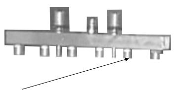
2. The oil hose is connected with the Oil Outlet on the Fuel injector distributor assembly.
