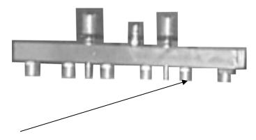
2. The oil hose is connected with the Oil Outlet on the Fuel injector distributor assembly.
