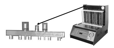
3. Fix the injectors that will be tested. First check the injector resistance value, this value can not exceed  $1\Omega$ , if the resistance value is above  $1\Omega$ , this injector must be replaced.
