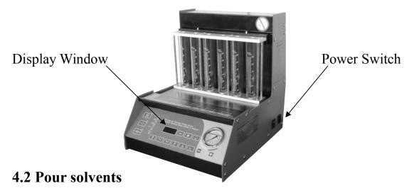
Pour suitable quantity of testing liquid into the unit from liquid inlet . If this unit is used for the first time, more than 2 L test liquid must be put into it. From the liquid level window, you can see the liquid level is above 6CLY. Do not mix the use of testing & cleaning solvents.
