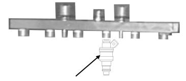
4.Please insert the pulse cable into the injector socket and mark the injectors in order.
