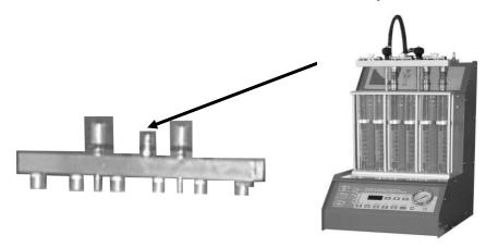
3. Fix the injectors that will be tested. First check the injector resistance value, this value can not exceed  $1\Omega$ , if the resistance value is above  $1\Omega$ , this injector must be replaced.
