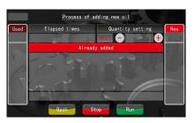
When the oil in transmission is not enough, supply it with the desired amount of oil. Select this operation. After adding the new oil, set the required oil amount in the interface and to run;
