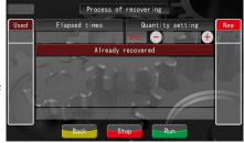
When the oil in transmission is too much, decrease it with the desired amount of oil. Select this operation.Set the required decreased oil amount in this interface, start the engine and to run;
