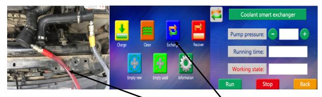
Start the engine. When liquid appears in the inlet hoseA start the machine. (Adjusted water pressure must be less than 0.1Mpa). Select exchange on the LCD screen. Click run (press +, - to adjust pump pressure). New/used coolant fluid exchanged realized between the engine and the machine.
