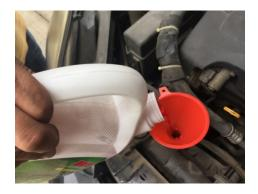
Fill the tank with coolant
