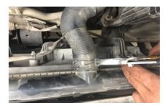
**R**emove the radiator upper pipe Choose the proper rubber hose from the toolbox
