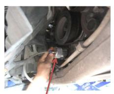
Tighten the combined adaptor on the oil filter seat
