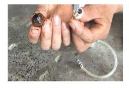
Choose appropriate adaptor from toolbox to screw on the oil pan drain hole
