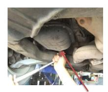
Remove the screw below oil pan
